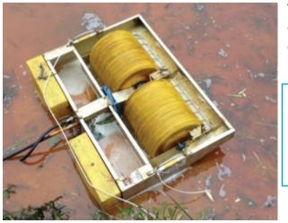
**TDS118 Drum Skimmer** is available in pneumatic or hydraulic drive for oil spill response or industrial use. Due to its shallow draft and light weight, this practical skimmer is ideal for cleanup in creeks, rivers and lakes. Brush and Disc versions are available.
