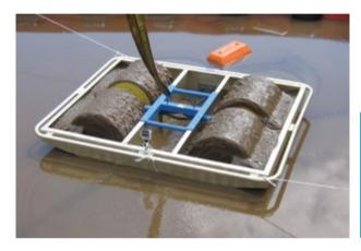
**Magnum 100 Drum Skimmer** is suited for larger spills in inland and coastal waters. The four drums provide more stability in open water, while an optional Wave Breaker increases the freeboard. Steam coils can be fitted for cold environments.
